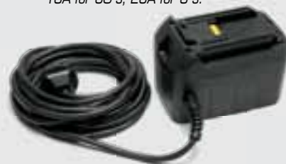
BPS 230.24 , network power supply. Main features: INPUT 230V~ 50-60Hz; OUTPUT 24V ~~~ thermal and short circuit protection. Current supply: up to 4A extended use; 18A for 50 s; 25A for 8 s.
